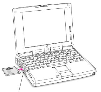
A Type III PC Card must be inserted in the lower slot.
